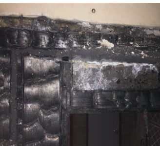
Graphite based intumescent after fire
