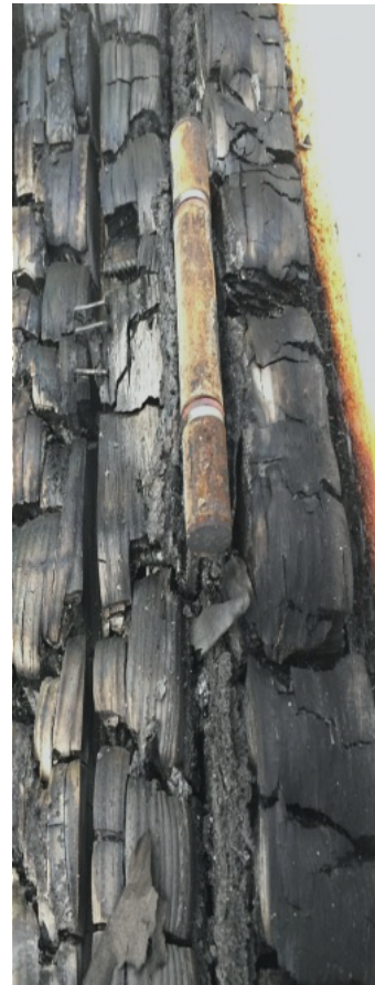
Graphite based intumescent seal once expanded
